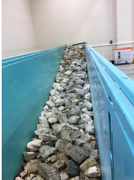
Figure 4.4 A wave breaking beach with 1/5 slope made by stones are placed at the end of the tunnel
