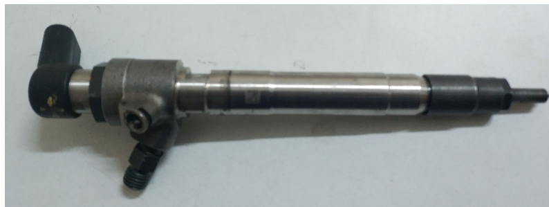
Figure 3.13. Piezoelectric injector used in the study.
