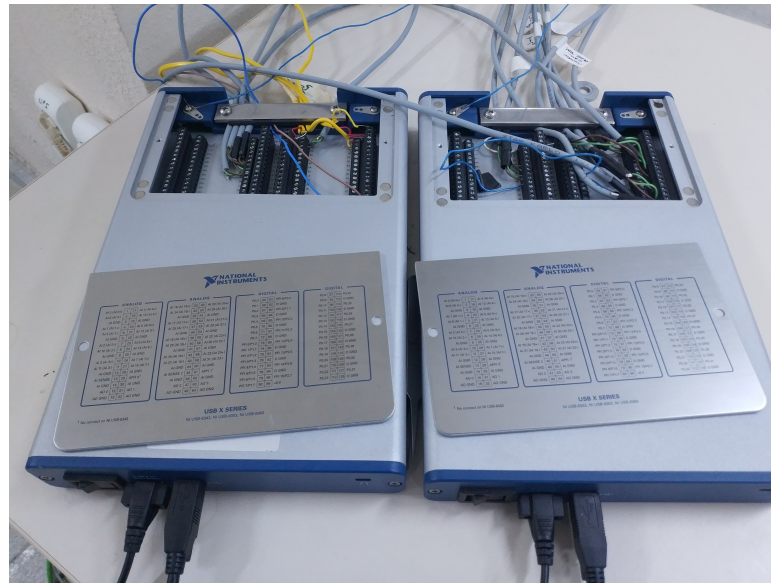
Figure 3.22. NI USB 6353 DAQ cards used in the study.
