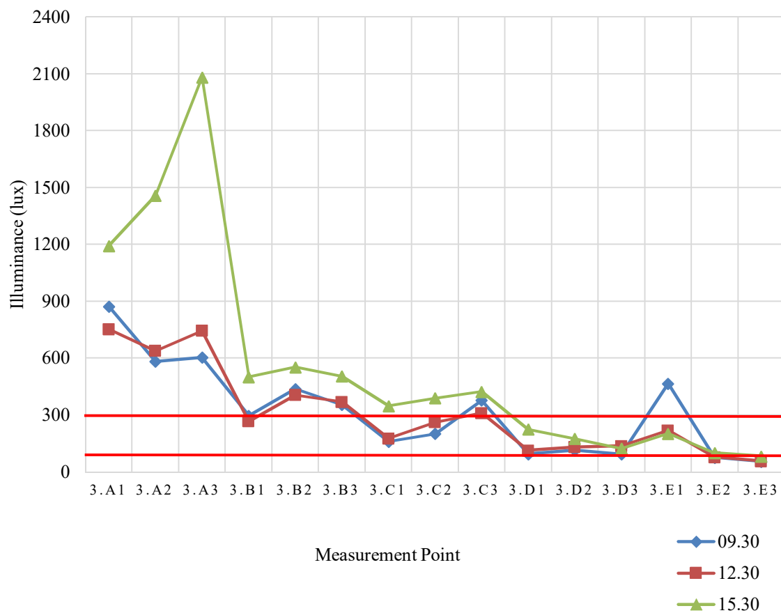
Figure 5.60. Measured interior illuminance (lux) (April 3, 2019)
