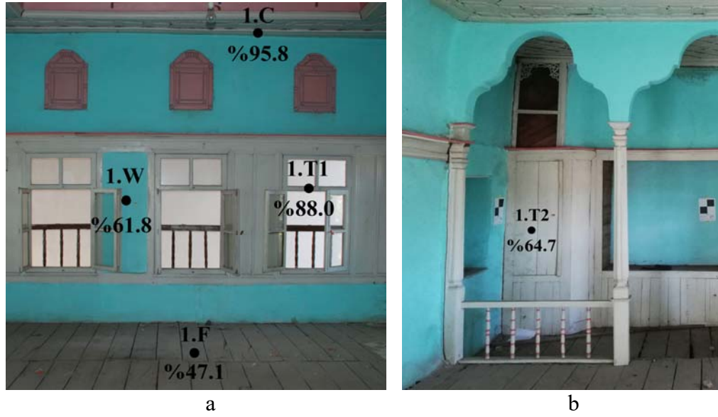
Figure 5.18. The surface reflectance at the measurement points in the main room of Kaçıklar House on the west wall (15.10.2018) (a), on the east wall (15.10.2018) (b).
