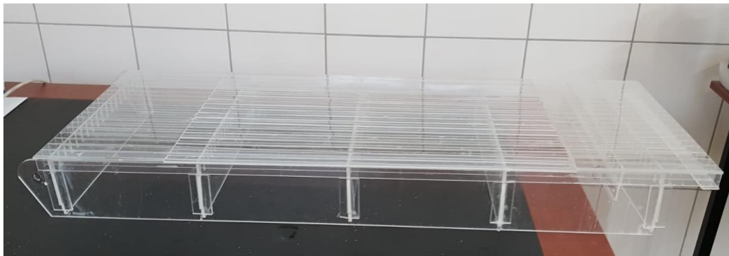
Figure 41. Example of the Tyrolean intake that is used in the experiments
