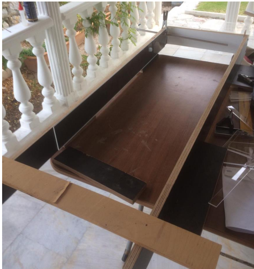
Figure 35. Wooden frame for constructing intakes
