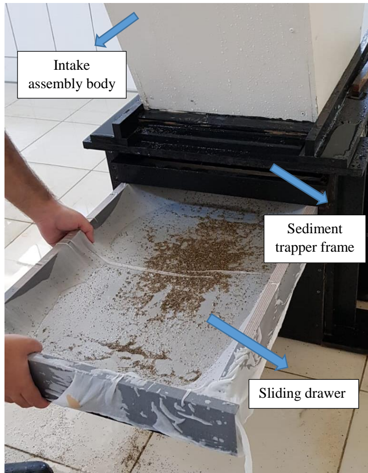
Figure 45. Sediment Trapper (Sliding drawer and its frame)
