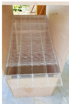
Figure 48. Intake assembly frame
