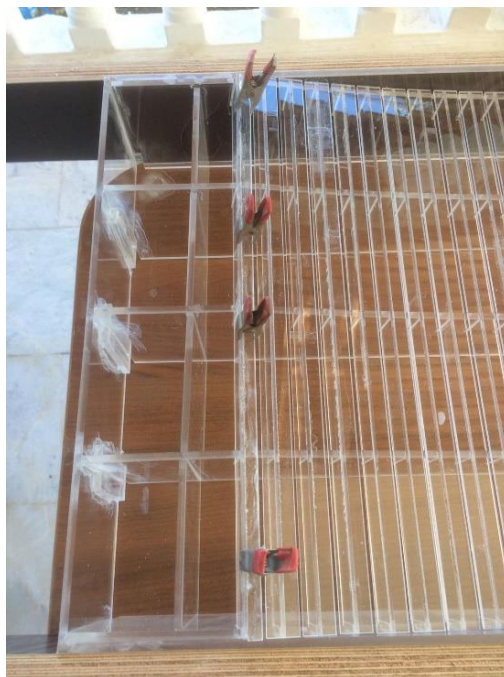
Figure 38. Fixing last T-shape bar on its position
