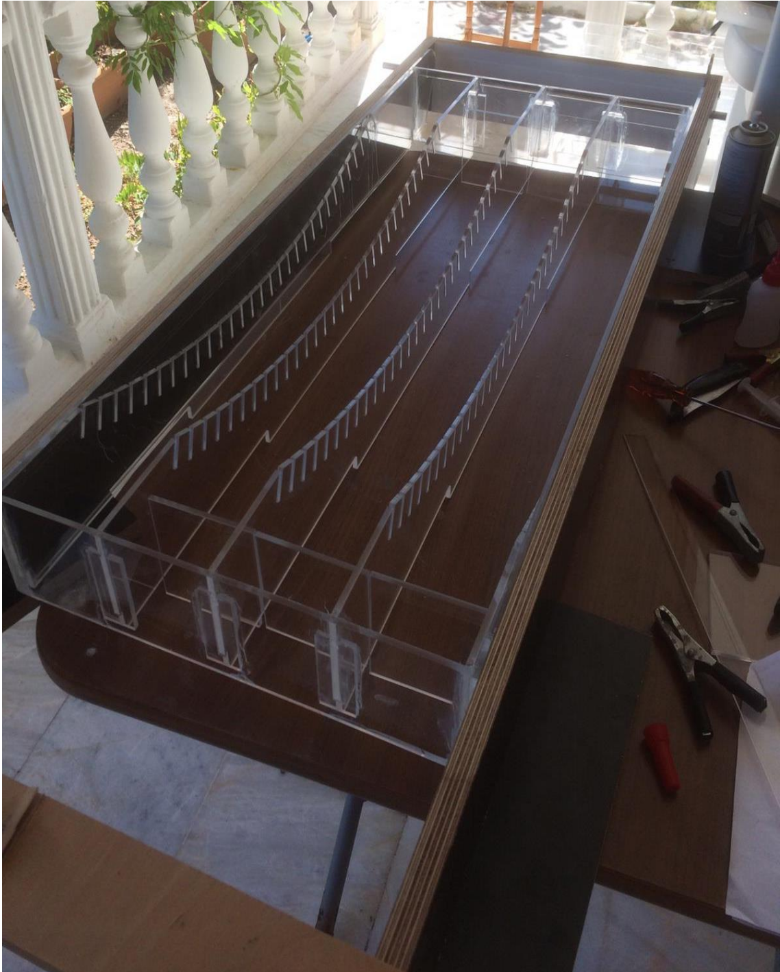
Figure 36. Assembly of middle parts to the Coanda screen model
