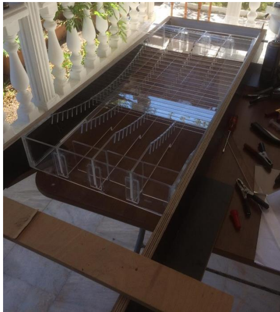
Figure 37. Fixing the T-shape bars in their positions on the model
