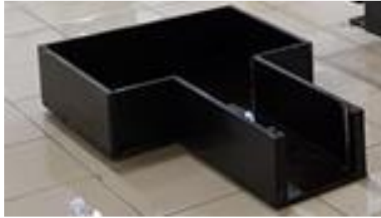
Figure 47. Flume for routing the downstream flow
