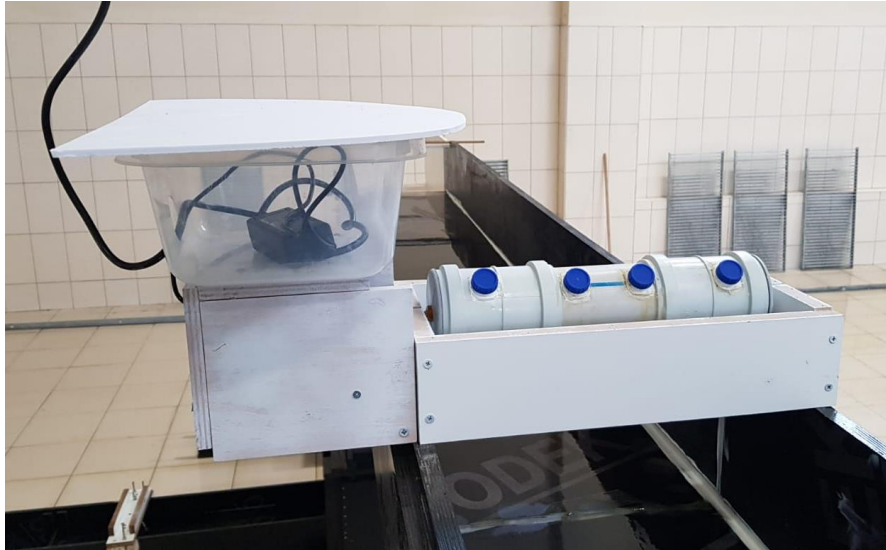
Figure 50. Sediment feeder device
