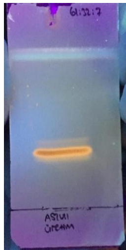
Figure 48. HPTLC profile of AST VII obtained from precipitation of [Fr: 51-79] (Normal Phase Silica Gel Plate, Mobile Phase; 61:32:7; \text{CHCl}_3 :MeOH:H _2\text{O} )
