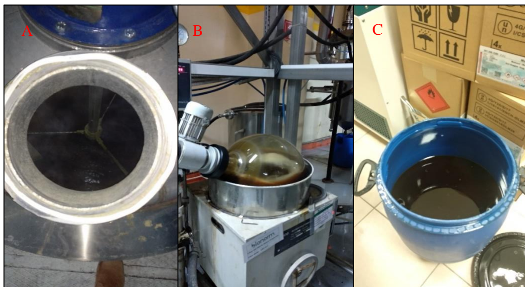
Figure 19. Photos of extraction; A) Top view of extractor, B) Evaporation, C) The crude extract
