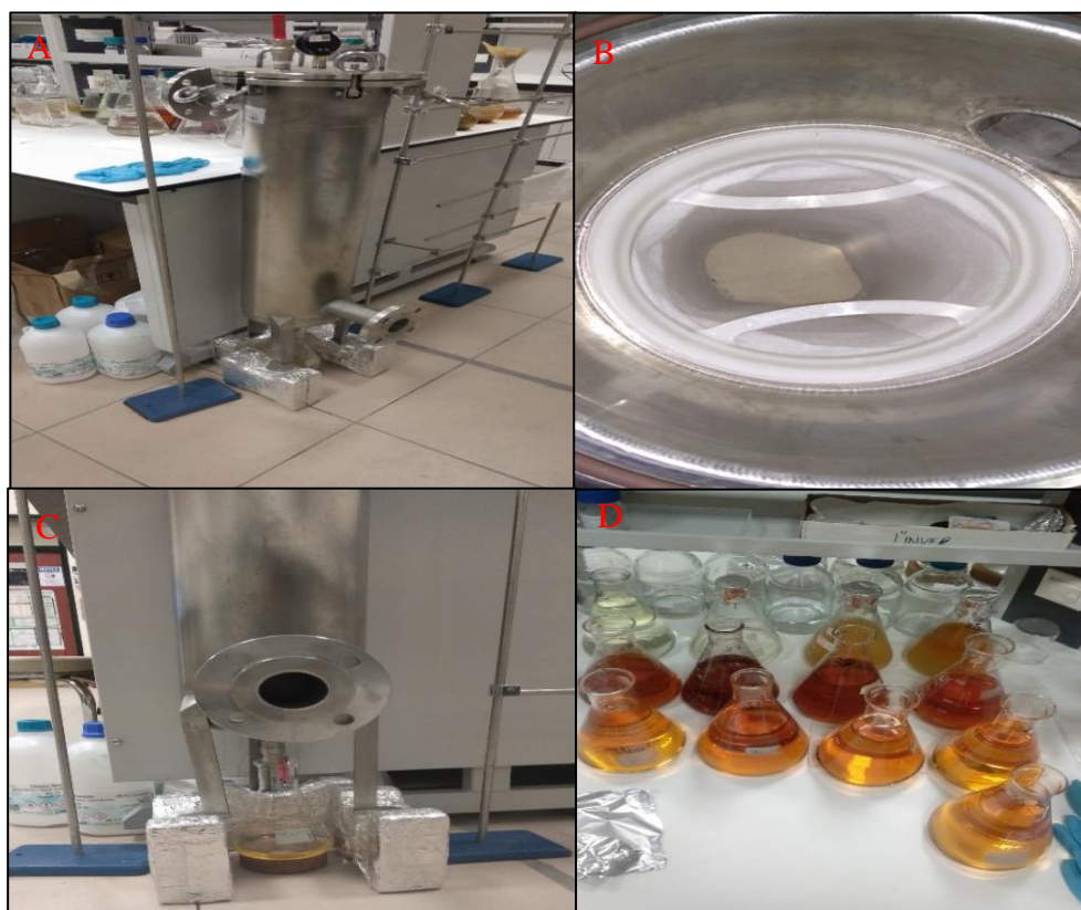
Figure 13. Photos of resin column; A) Single bag filter container as a column, B) Top view of column, C) Fraction collection, D) Saponin rich fractions
