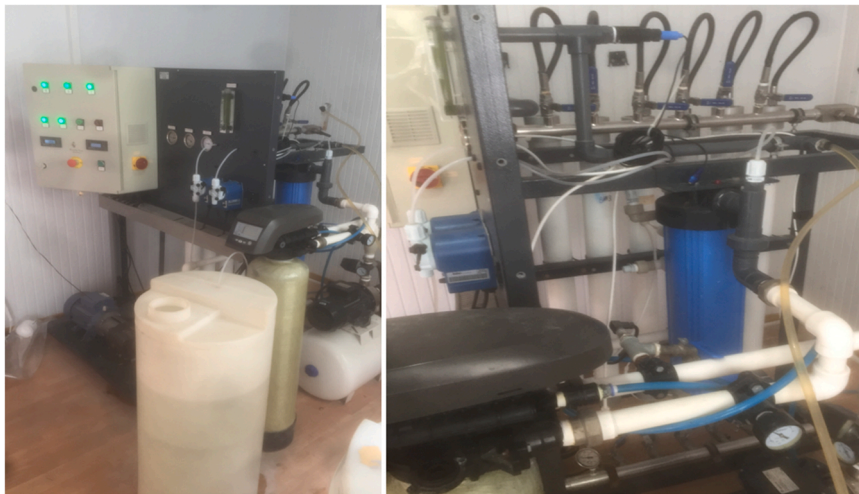
Fig. 3. Mini-pilot scale membrane test system front view (left), side view (right).
