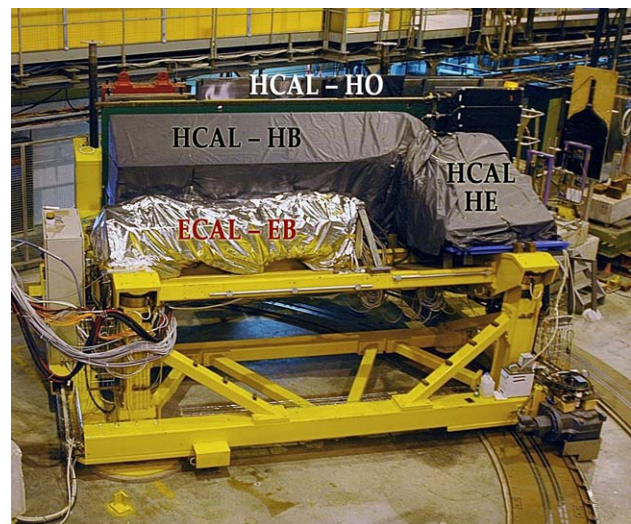
Fig. 2.1 The ECAL and the HCAL modules on a moving platform in the CERN H2 test beam area. The transporter table which supported the wedges is designed to move in \phi and \eta directions, approximately 0 to 30^\circ in \phi and 0 to 3.0 in \eta
