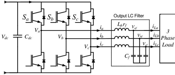
Fig. 1. Inverter with an output LC Filter
