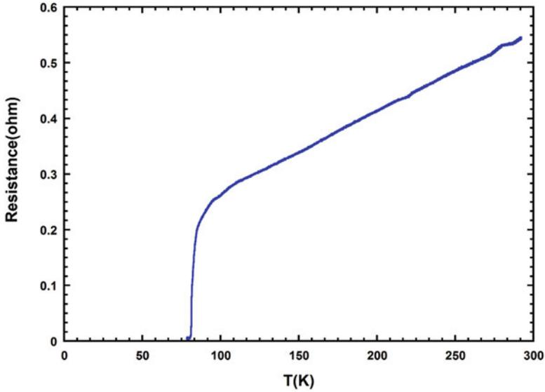
Fig. 11.3 Temperature dependence a-b axis resistance behavior of one of the fabricated Bi2212 microchip
