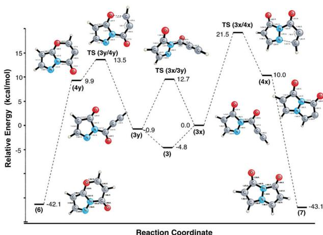
**Fig. 5** Potential energy profile related to the formation of the products, intermediates and transition states. Energies of structures **3**, **6**, and **7** are computed relative to  $3x + H$ , since they have different stoichiometry.
