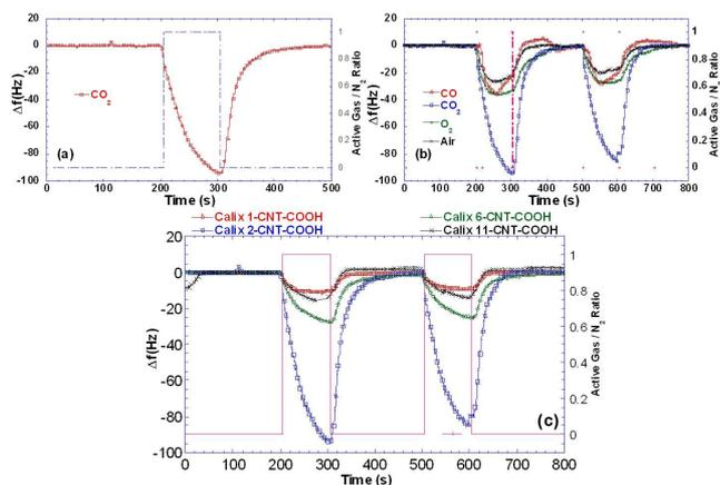
Fig. 4. QCM frequency shift of: (a) calix 2 modified CNT films for adsorption and desorption cycles under CO<sub>2</sub>, (b) calix 2 modified CNT film under different gases, (c) various calixarene molecules modified CNT films under CO<sub>2</sub>.
