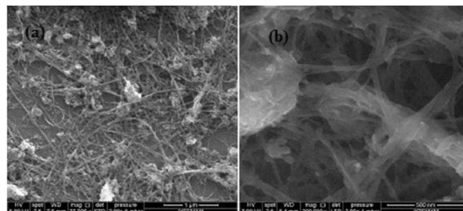
Fig. 3. SEM images of calix[4]arene modified SWCNT-COOH structures.
