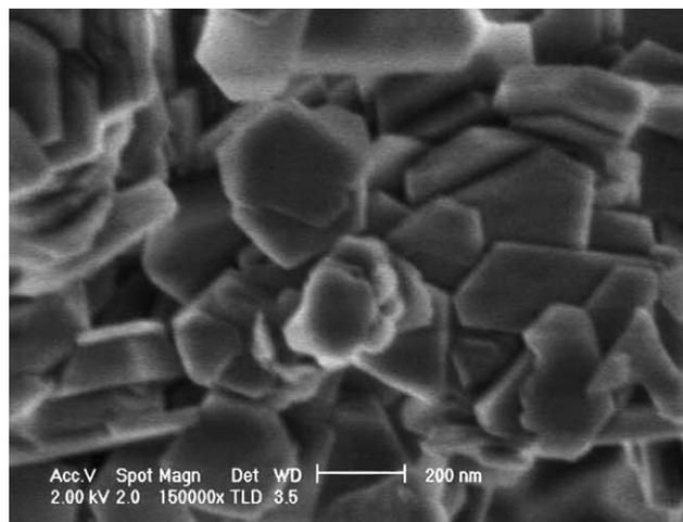
Fig. 2. SEM micrograph obtained at  $\times 150,000$  magnification for the natural kaolinite used in this study.
