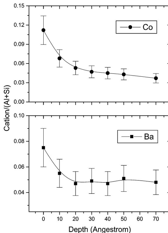
Fig. 4. Variation of the sorbed amounts (cation/(Al+Si)) of  $Ba^{2+}$  and  $Co^{2+}$  with depth (Å) in kaolinite lattice. The fits are used to guide the eye.
