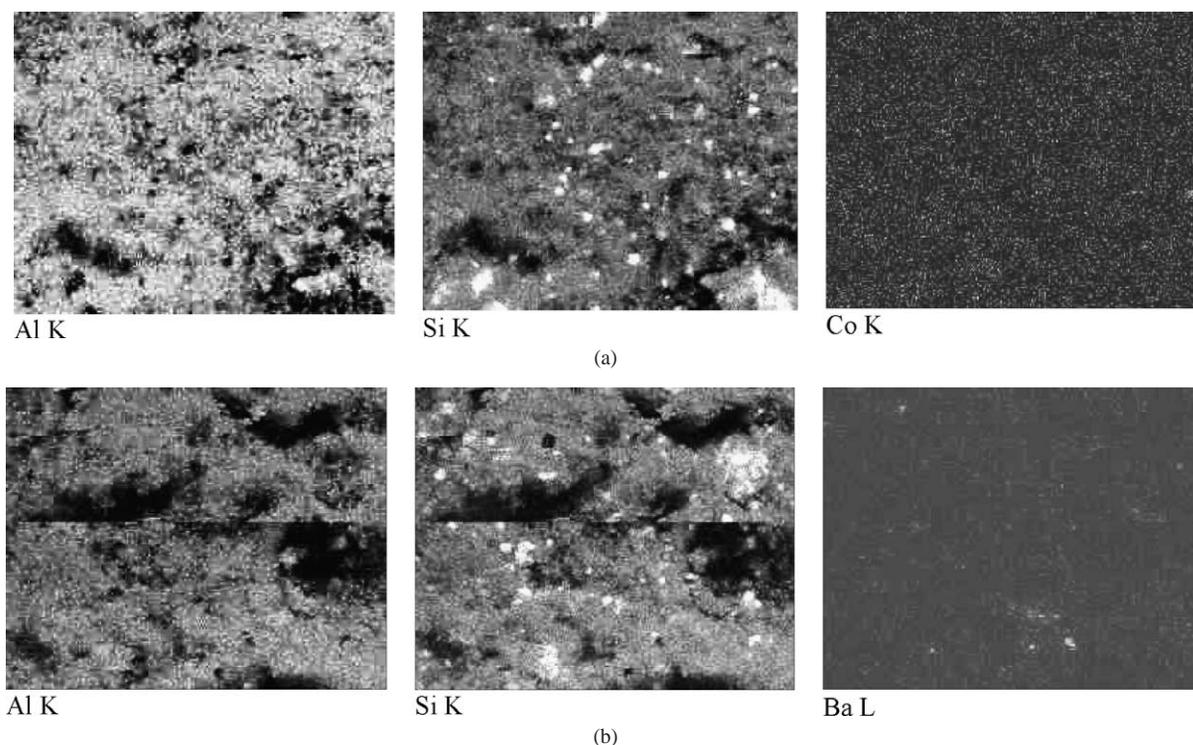
Fig. 5. SEM mapping images of Al, Si, and Co or Ba in (a) Co-sorbed kaolinite and (b) Ba-sorbed kaolinite.
