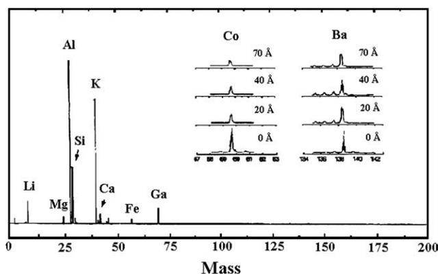
Fig. 3. A typical ToF-SIMS spectrum of the clay sample before sorption. The insets show the variation of sorbed Ba<sup>2+</sup> and Co<sup>2+</sup> signals on the clay at different depths.
