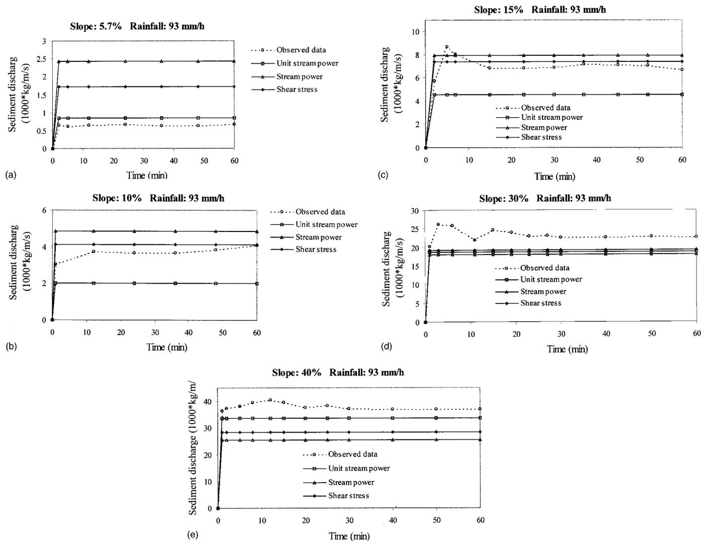
**Fig. 3.** (a) Simulation of observed data; ( $S=5.7\%$ ,  $r=93$  mm/h); (b) simulation of observed data; ( $S=10\%$ ,  $r=93$  mm/h); (c) simulation of observed data; ( $S=15\%$ ,  $r=93$  mm/h); (d) simulation of observed data; ( $S=30\%$ ,  $r=93$  mm/h); and (e) simulation of observed data; ( $S=40\%$ ,  $r=93$  mm/h)
