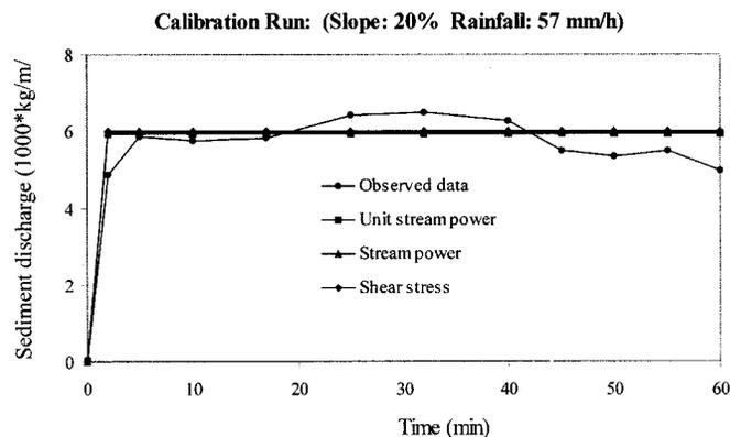
Fig. 1. Simulation of observed data; calibration run ( $S=20\%$ ,  $r=57$  mm/h)
