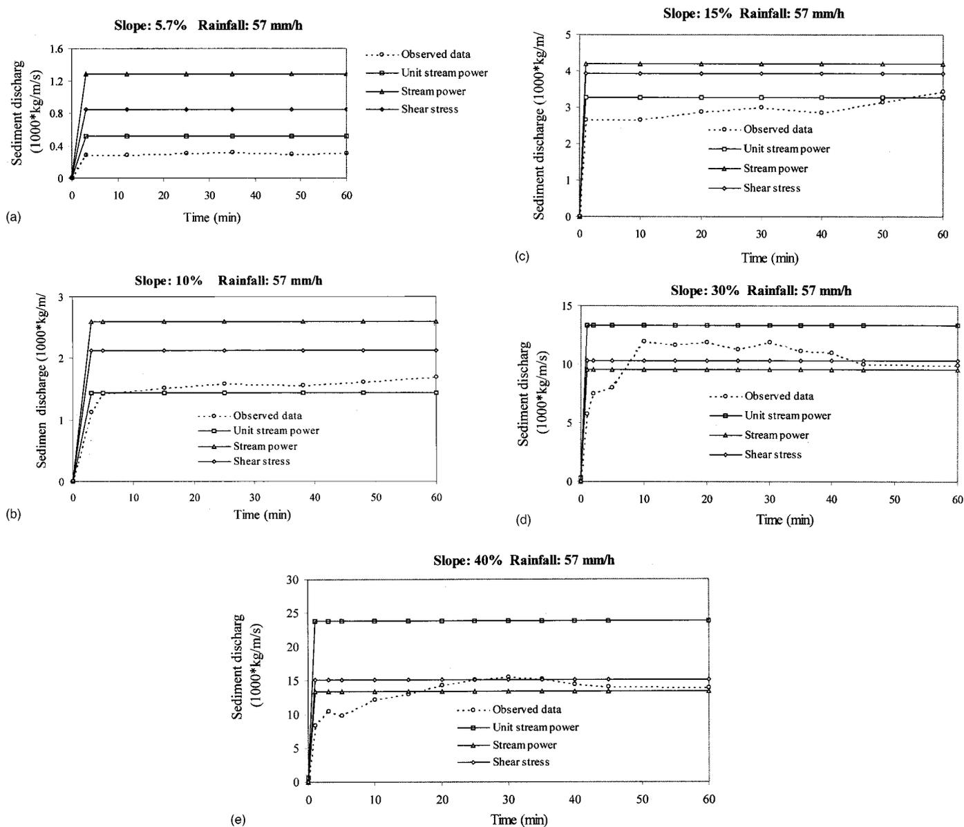
**Fig. 2.** (a) Simulation of observed data; ( $S=5.7\%$ ,  $r=57 \text{ mm/h}$ ); (b) simulation of observed data; ( $S=10\%$ ,  $r=57 \text{ mm/h}$ ); (c) simulation of observed data; ( $S=15\%$ ,  $r=57 \text{ mm/h}$ ); (d) simulation of observed data; ( $S=30\%$ ,  $r=57 \text{ mm/h}$ ); and (e) simulation of observed data; ( $S=40\%$ ,  $r=57 \text{ mm/h}$ )
