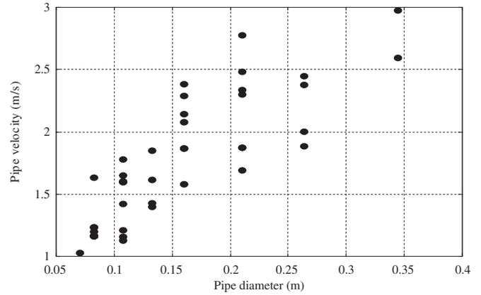
Fig. 7. Relationship between pipe diameter and velocity of water.
