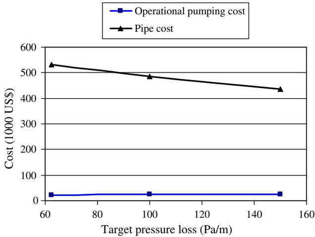
Fig. 5. Operational pumping and pipe cost for the network.
