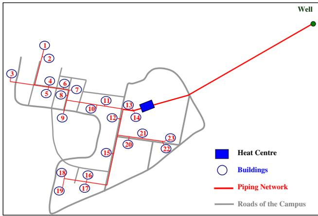
Fig. 4. District heating piping network: Alternative 3.
