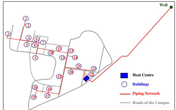
Fig. 2. District heating piping network: Alternative 1.
