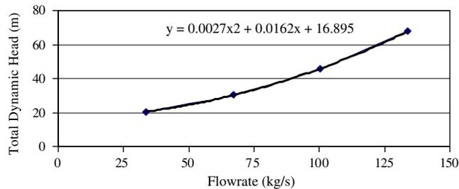
Fig. 10. Variation of total dynamic head of the geothermal loop circulation pump depending on the geothermal fluid flowrate.
