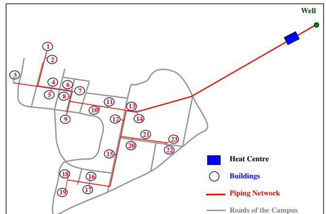
Fig. 3. District heating piping network: Alternative 2.
