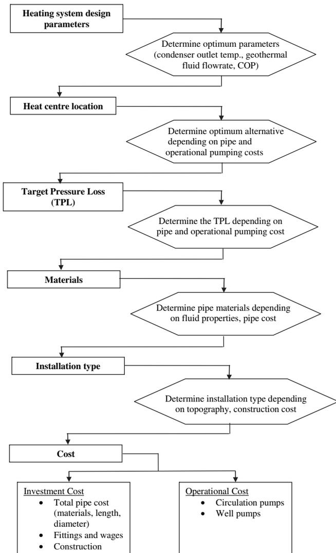
Fig. 1. Flow diagram of piping network design.
