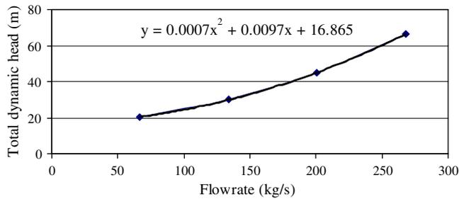
Fig. 9. Variation of total dynamic head of the campus loop circulation pump versus secondary water flowrate.
